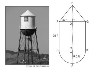
If AC = 8.5 feet, BF = 25 feet, and  $m \angle EFD = 47^\circ$ , determine and state, to the *nearest cubic foot*, the volume of the water tower.
